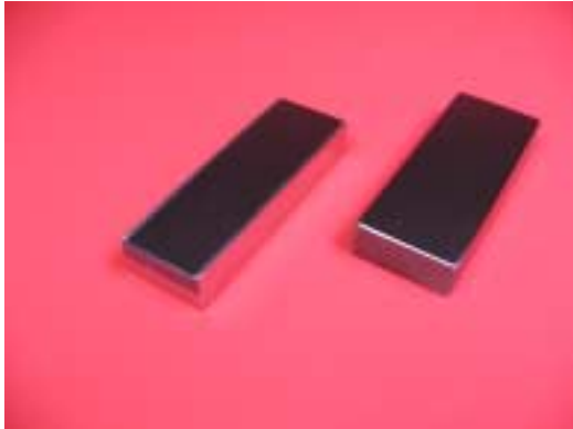
Fabrication of high precision 60 mm parallel beam optics both on prefigured substrates (right) and on flat substrates, which are glued and bend after deposition (left)
