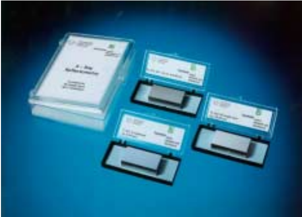
Teaching tool for X-ray reflectometry: pure silicon substrate, Ni-single layer, 10 period- Ni/C-multilayer
