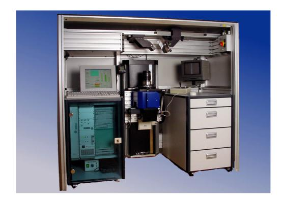
The **modulation transfer function (MTF)** is since many years an established concept to describe the image quality of lenses. It's fast and simple measurement is an indispensable tool in industrial and application oriented laboratories.
