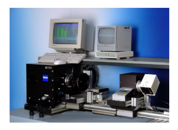
The Modulation Transfer Function (MTF) of lenses is a generally accepted criterion to define the optical performance of a lens. Evaluating MTF is a powerful tool to check several lens parameters.
