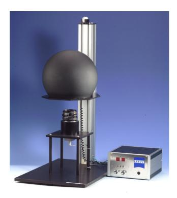
The Carl Zeiss **T-Stop Tester** is an universal, modular designed test equipment for measuring **apertures** of **photographic lenses**.
