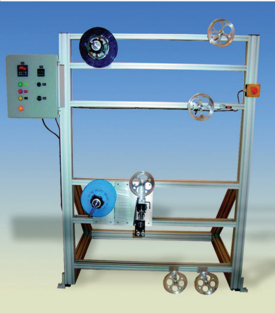
This fiber optic wire spooler was custom built to perform in a customer's coating process. It accommodates oversize spools that are 300mm long and 1 meter in circumference. Using a closed-loop speed control system, the fiber travels very slowly and steadily; and the guide rollers were custom made to provide absolutely straight travel with little or no vibration. Finally, the machine's frame was custom designed to accommodate special coating equipment supplied by the customer.
