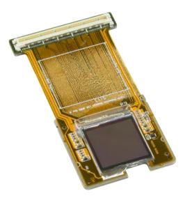
No sub-pixels, customisable colour gamut, no image burn-in of static content and fast refresh make the 2K microdisplay particularly suitable for applications requiring high fidelity images. Optional ancillaries include a LED driver and a low profile RGB LED illuminator. ForthDD's highly experienced engineering support will shorten your design-in time.
