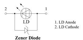
This model does not have a Photo Diode. This model has a Zener Diode built in as a protection circuit against static electricity.
