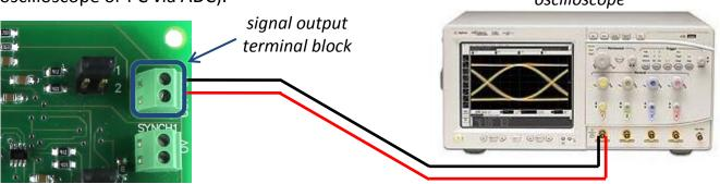
4. Connect wires from LED driver's synchronization output with synchronization input terminal block (7).
