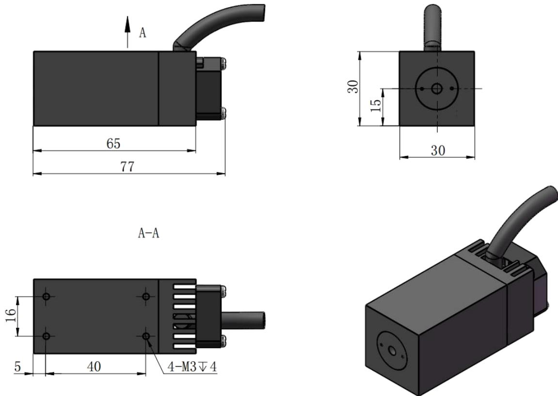
Dimensions of PSU-V-OEM power supply
