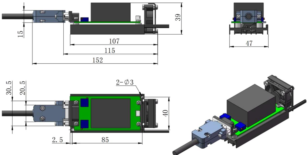
Dimensions of PSU-I-OEM power supply(107×47×38mm<sup>3</sup>, 5/12VDC, TTL 30kHz and Analog 0-5V)
