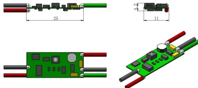
Dimensions of external PCB2(*wide voltage input range*, $20 \times 30\text{mm}^2$ ,5-12VDC,TTL and Analog)
