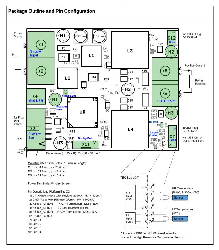
Peltier element, temperature probes, power supply and connectors not included.
