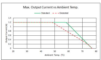
Standard or Extended Device Temperature Mode can be set as software setting.
