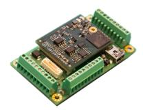
Status information can be polled at any time by industry standard RS485 / RS232 TTL connection or by USB (see box below). The TEC-1092 can also operate in a remote-controlled manner, with parameters adjusted on the fly. Scripting capability by sequential lookup table read-out is supported.
