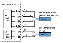
\* The TEC-1092 always uses 4 wires to sense the High Resolution temperature. There are no bridge jumpers on board. For NTC, please make a bridge on the mother board close by the X1 connector.
