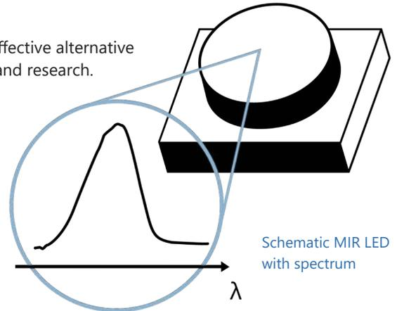
Schematic MIR LED with spectrum
