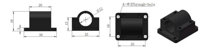
This simple mount acts as combined heat sink, electrical insulator mount for 12mm diameter diode modules. Loosen the four small set screws and remove the top half of the module mount to put the laser in. The laser is held firmly by tighten the screws. The module mount reserved 4 through-holes for user to fix the laser on a flat and thermally dissipating surface.
