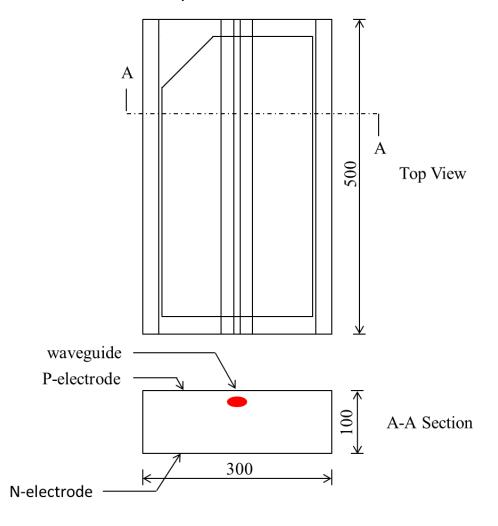
O P-electrode and N-electrode are both gold pads.
