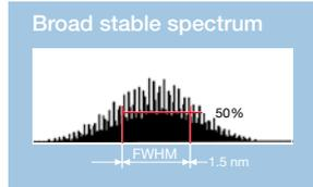
Broadened spectrum (~1.5 nm FWHM) with reduced coherence length (~0.3 mm) as a result of RF modulation. No mode hopping occurs.
