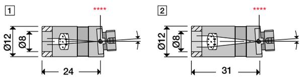
\*\*\*\* Additional grub screw for locking of the fiber ferrule (FC and LSA only)
