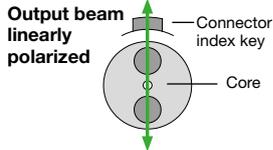
Axis orientation of a polarization-maintaining fiber with the connector key
