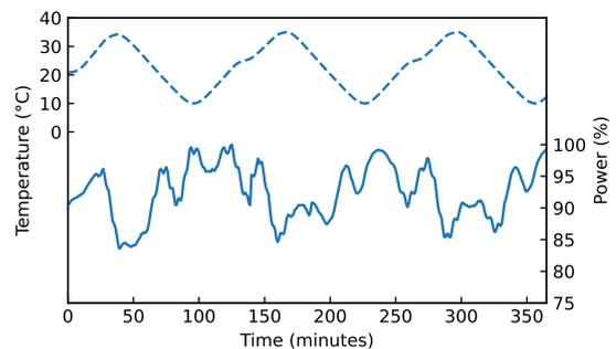
The ambient temperature is varied between 10 °C and 35 °C in a climate chamber with a cycle time of roughly 130 minutes (dashed line). Measured relative output power of the fiber-coupled double-pass AOM as a function of the cycling time (solid line). (all values and data are preliminary)
