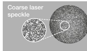
The laser spot produced by a standard laser diode beam produces a speckle pattern, increasing the statistical uncertainty in position determinations.
