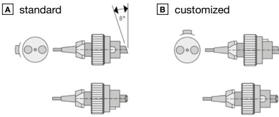
Orientation of the 8°- polish and index key for fiber connectors of type FC-APC:
