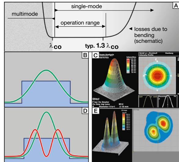
Operating range of a single-mode fiber [A] Gaussian mode field of a single-mode fiber [B] and resulting Gaussian intensity distribution [C] at the fiber exit.
