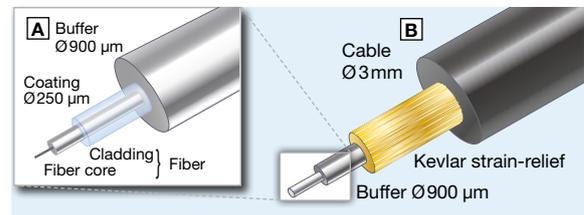
900  $\mu\text{m}$  buffer cable [A] or 3 mm cable [B]
