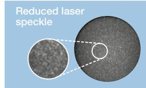
Low speckle contrast from reduced coherence length: uniform illumination of 4-quadrant diodes with improved position detection, e.g., in AFM.
