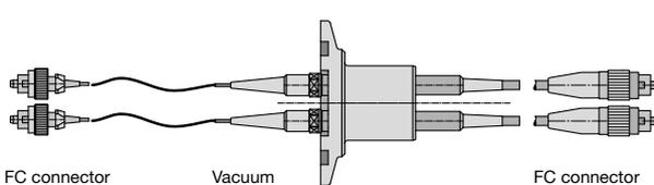
Flange type KF50 available with 1, 2, 3, or 4 fiber cables of arbitrary type
