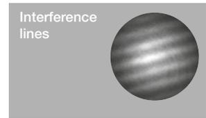
Collimated laser beam recorded directly using a flat camera sensor, with its protection window generating a disturbing pattern of interference.
