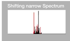
Mode hopping: temporal shifts between modes. The coherence length changes over time. It can be > 1 m.
