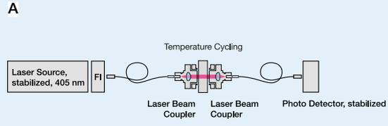
**Test setup for measuring the stability of two laser beam couplers ( $f = 4.5 \text{ mm}$ ,  $\lambda = 405 \text{ nm}$ ) during successive temperature cycling between 15 °C and 35 °C (A).**
