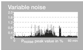
Stochastic power noise resulting from, for example, an external cavity between the laser diode and its fiber coupling.
