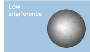
The Gaussian intensity distribution of the collimated laser beam on a flat camera sensor. Despite the sensor protection window, there are no interference patterns.
