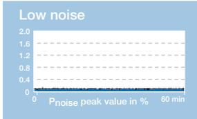
With RF modulation, mean laser power is constant with noise typ. <math>< 0.15\%</math> of  $P_o$  (RMS, Bandwidth <math>< 1</math> MHz).
