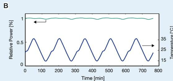
The repetitive pattern in the relative power caused by the temperature cycling is demonstrated more clearly in Fig. C, in which the relative power (normalized to the maximum) is plotted against the temperature of the laser beam couplers.
