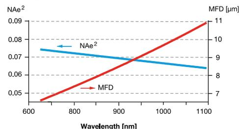
Typical wavelength dependency: Effective numerical aperture  $NAe^2$  (left scale) and mode field diameter  $MFD$  (right scale) as a function of the wavelength for a PMC-780 fiber.
