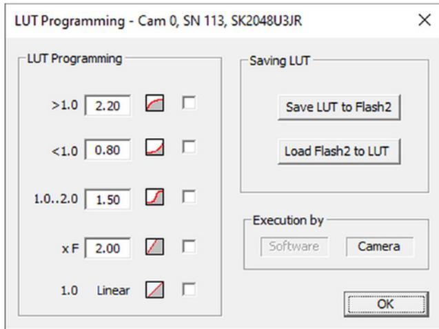
The Lookup Table (LUT) within the camera can be used for pre-processing the signal data. By programming a transformation function, brightness values of the camera can be converted to their corrected values. The transformation of image data can be useful in obtaining better imaging results, such as providing more contrast or higher dynamic range.
