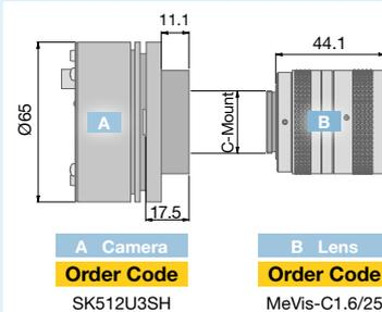
The Schäfter+Kirchhoff line scan cameras which can be used with C-Mount lenses have a corresponding female C-Mount (1"/32 TPI) thread.
