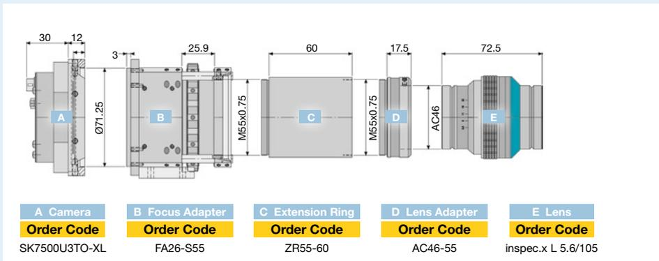
Scan and macro lenses require a focus adapter for focusing and one or more additional extension rings. Depending on the lens mount (V-Mount in this example), additional lens adapters may be necessary. Extension rings, the focus adapter, and the lens adapter together provide the tube length LT (see page 53, F4):
