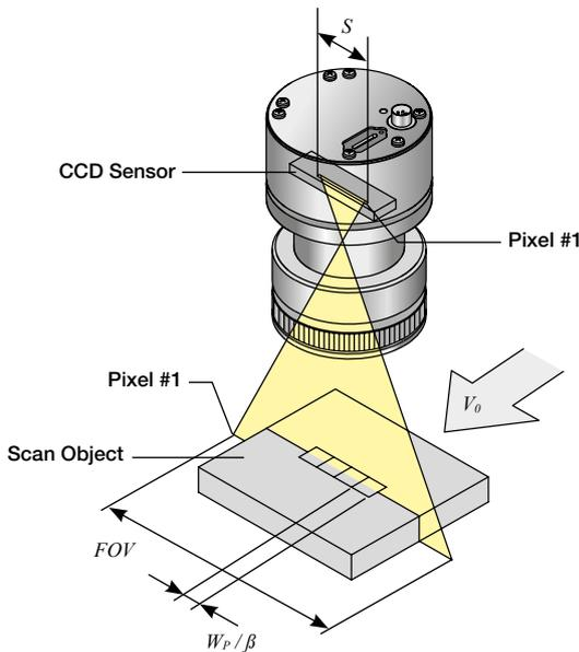
The native resolution of an optical line scan camera is defined by the number of pixels – the row of photosensitive elements in the sensor line. Line scan cameras are available with more than 8000 pixels.
