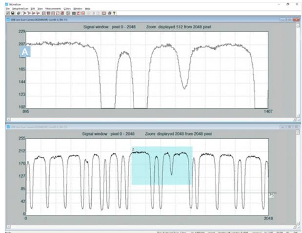
Control of the camera integration time and setting of line frequency. **A**
