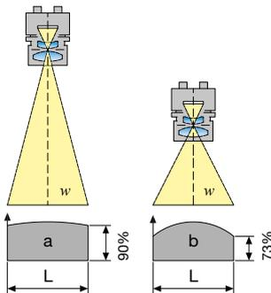
**Example:** Edge intensities calculated for two different field angles using the same sensor length  $S = 28.7$  and magnification  $\beta = 0.25$ :
