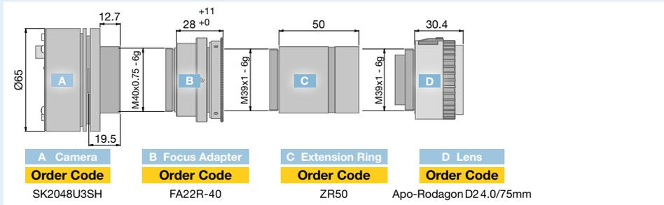
Scan and macro lenses require a focus adapter for focusing and one or more additional extension rings. Extension rings and the focus adapter together provide the tube length LT (see page 53, F4):
